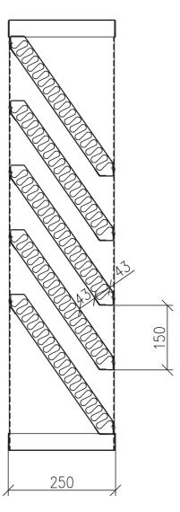
IAS jalousie silencers are the elements which constitute an acoustic barrier and enable air flow at the same time. They can be applied as the element of the IAS acoustic enclosures, vents' shielding of the spaces where noise emitting devices are located or as individual acoustic screens around the noise sources that require a constant air flow.
